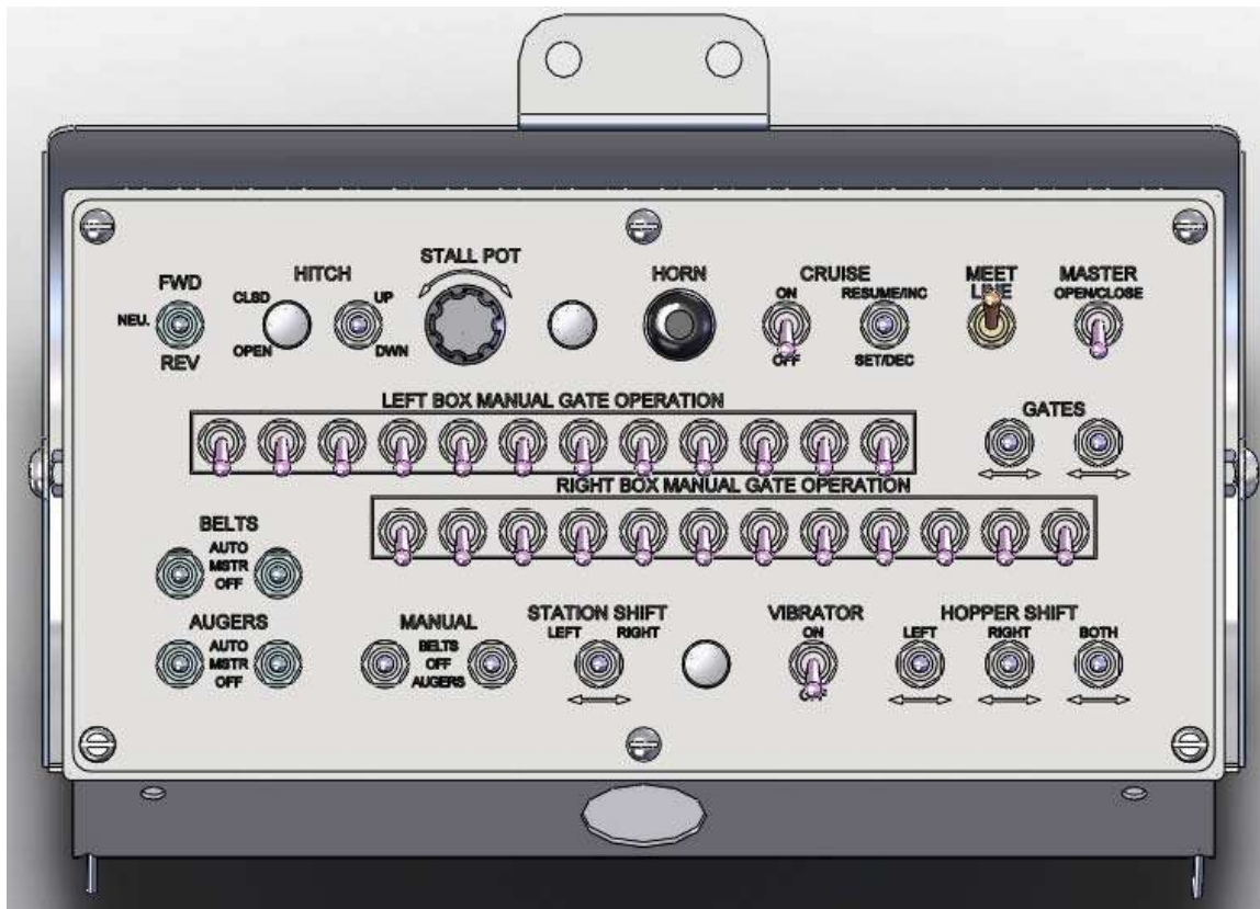
Figure 3-3. Control panel switches 2008 & up
