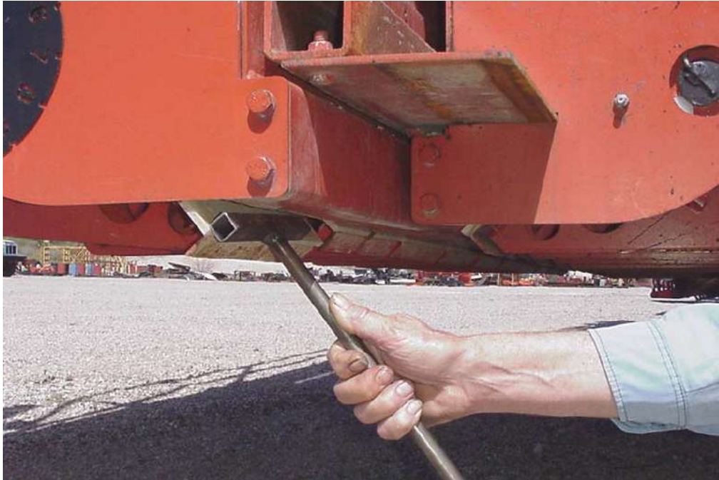
Figure 6-2. Checking Gate Opening
